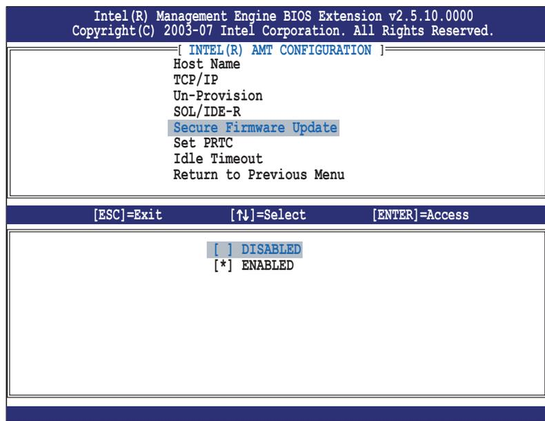
**Figure 16.6** Intel® MEBX Option to Enable or Disable Secure Firmware Update
