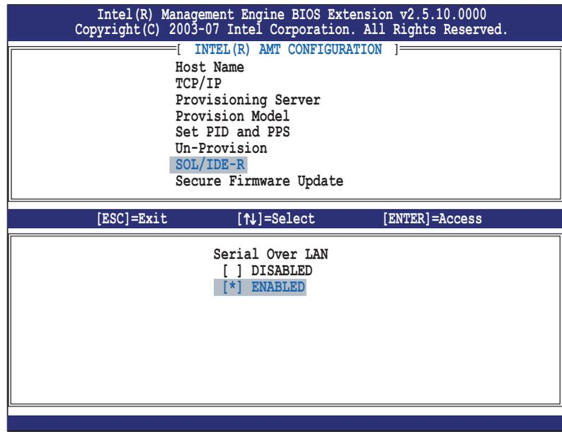
**Figure 16.4** Intel® MEBX Option to Enable or Disable Serial over LAN
