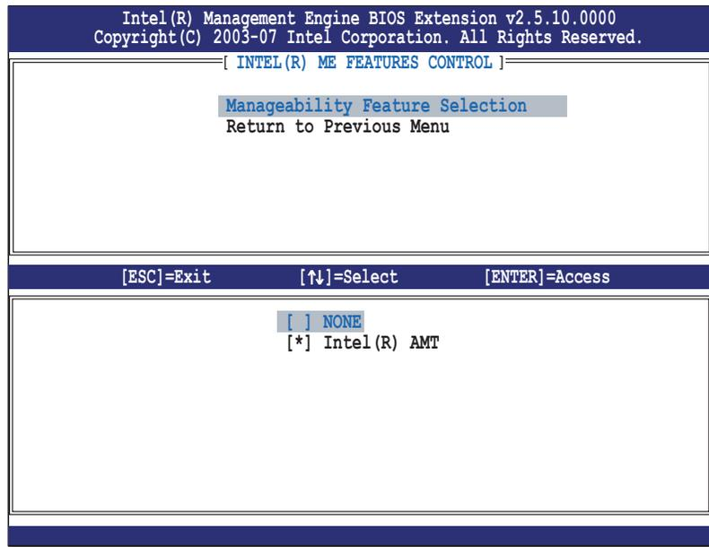
**Figure 16.2** Intel® MEBX Option to Enable or Disable Intel® AMT
